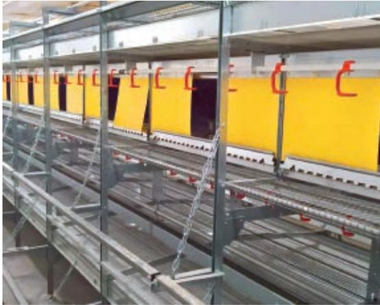
The All-In-One aviary system has been developed as a bird friendly, high performance system resulting in the maximum number of sellable eggs. It's available in different widths (2000 & 2400 mm) to allow optimum use of the house and optimum stocking density.
