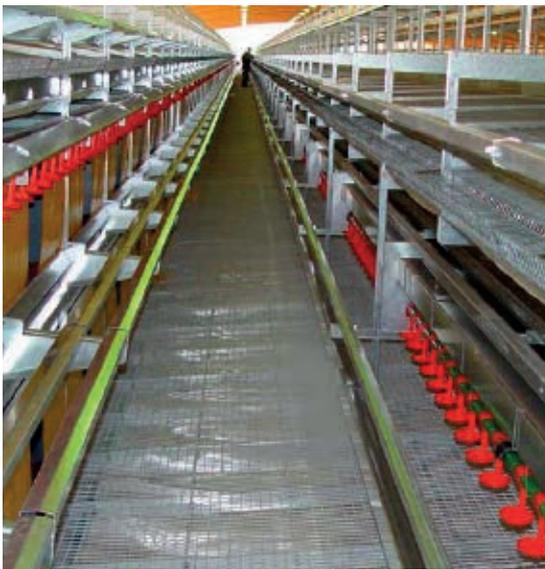
Nests, feed, water, perches and slatted area are easily reachable by the birds. The slope of the floor towards the nest makes sure the eggs roll into the nest to avoid having eggs visible in the system. Perches in front of the nest can be lifted creating more space for catching and cleaning.
